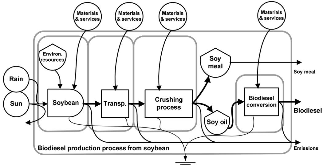
Figure 1: Energy system diagram of the biodiesel production process from soybean.
