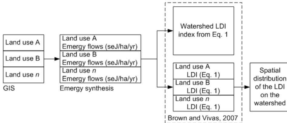
**Figure 1.** Flowchart for LDI index calculation in this paper.
