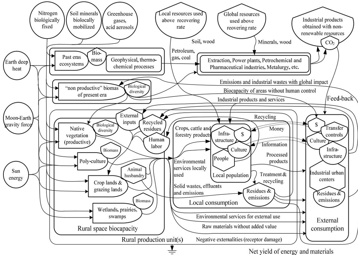
**Figure 6.** A systems diagram that shows four critical relationships of agriculture: (a) with other Era’s ecosystems areas (fossil fuel); (b) with present era “non productive biomes” whose preserved areas provide Biosphere functions (climate regulation); (c) clean development mechanism areas needed for CO<sub>2</sub> sequestering; (d) internal complexity of rural space biocapacity and local consumption.
