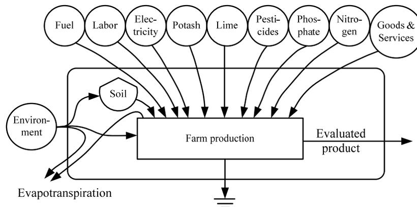
**Figure 1.** Systems diagram with 11 inputs and 1 output applied to 22 crops (*Emergy Folio 4*).
