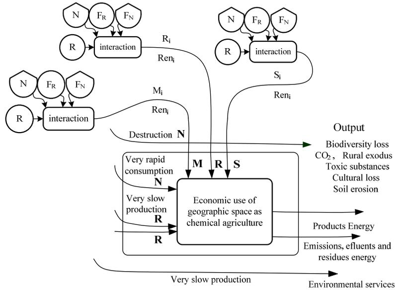
**Figure 4.** Aggregated flows diagram. If only cropland is considered (the small window) then the output corresponding to remaining environmental services and system losses will be excluded.
